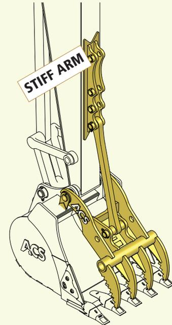
The **Direct Connect Hydraulic Thumb** is supplied with a heavy duty hydraulic cylinder. The rod-end of the cylinder mounts directly to the thumb body. The base-end of the cylinder mounts to a bracket (provided) that is welded to the underside of the machine stick. A hydraulic thumb allows the operator more flexibility in moving material towards the bucket and improves productivity and job safety by eliminating manual adjustment.
